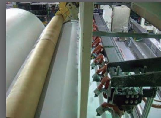
*Valves in the spray position mounted behind dust wall just before spray trigger*
