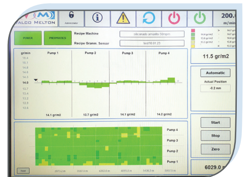
Weight Inspekt grammage control working in close-loop
