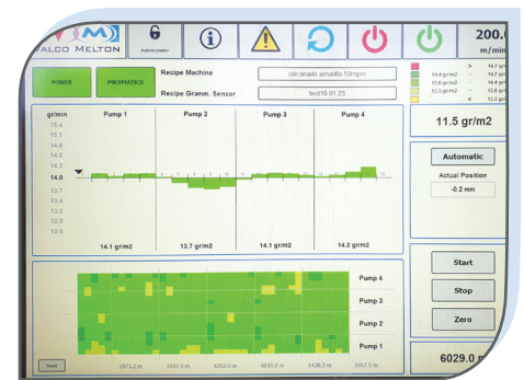
Weight Inspekt grammage control working in close-loop
