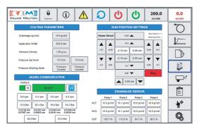
When working with our LP Series Coating Lines, or Akura Coating Stations, the system records the working parameters defined on the recipe for each roll produced. This information is stored along with the adhesive distribution map.
