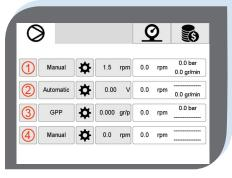
The pump control can be programmed in grams per product or grams per square meter, depending on each application's specific requirements.
