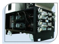
Reduce space on the floor with its compact design as the motors are vertically stacked in pairs
