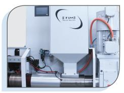
A water cooler system prevents clogging in the feeding area (Optional feature)
