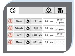
The extruder control is accessible through a user-friendly PLC touchscreen. Different standard fieldbus communication interfaces available
