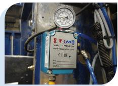
Automated air pressure adjustment stabilizes corrugated boards for smooth operation.
