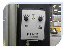
Ensures repeatable and precise flute height adjustment control for consistent glue application.
