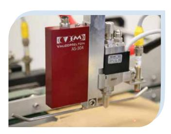
The AS-304 and 524 LNLR can be connected to the MCP-8i for gluing control and inspection.
