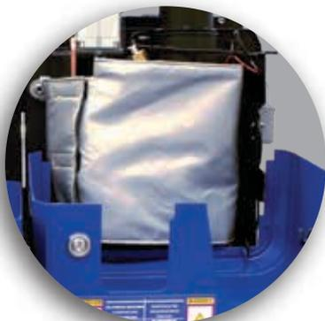
Protective cover provides a safer working environment while ensuring easy access to all components
