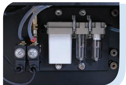
Dry air blanket prevents moisture from reaching the adhesive.
