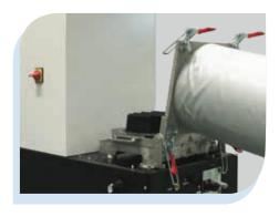
Its tiltable tank and removable melting grid facilitate maintenance and cleaning operations, which may be carried out faster and safer.
