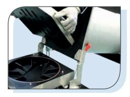
The reservoir tank eliminates production stops, even during PUR slug changes. New grid design with cast-in heaters for a more efficent melting process.
