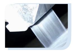
Adhesive is delivered through a central shim which provides the best protection against adhesive strikes-through when used to bond very thin substrates.
