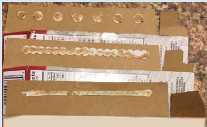
EcoStitch 点胶 VS 传统线状喷胶
