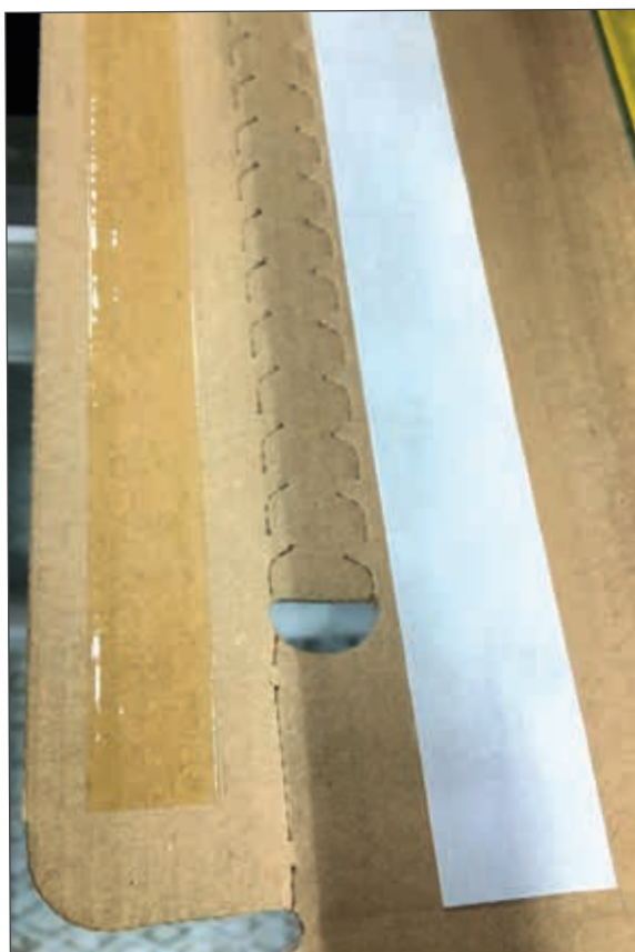
High precision hot melt cut off ensures a clean process without angel-hair build up
