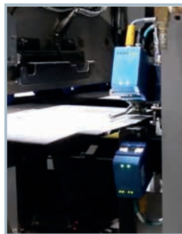
Double camera installation for back side inspection
