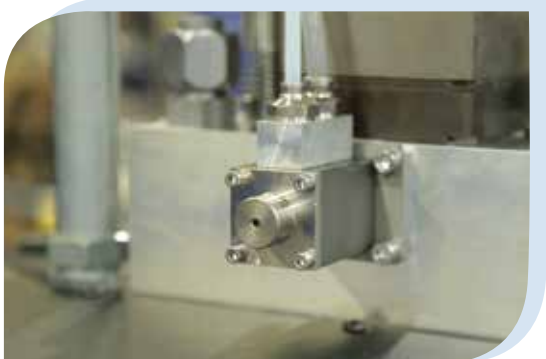
Automated blow-off valve safely regulates internal drum pressure during changes
