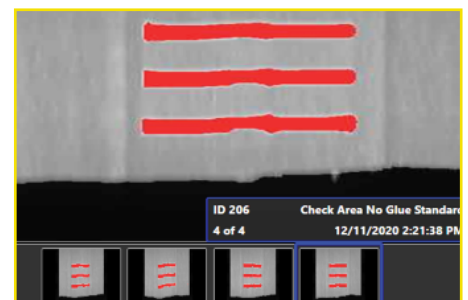
No Glue Defect
