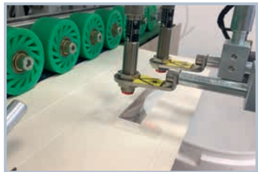
The system can be equipped with 2 or 3 photo-eyes.
